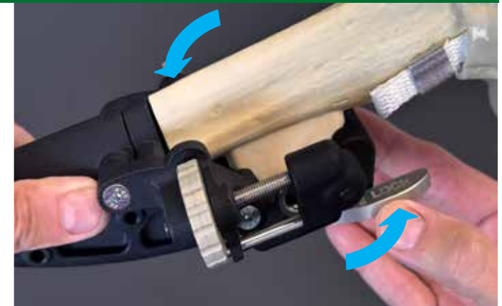
... then push the notch into the Notch Holder and engage the locking lever
