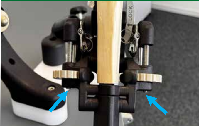
Ensure that the end of the tensioner spindle is flush with the housing before securing the ligaments. If necessary, turn the wheels clockwise to achieve this.
