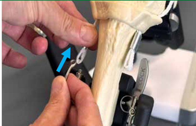
Open the snap shackle by pulling the ring and pass the shackle arm through the ligament loop...
