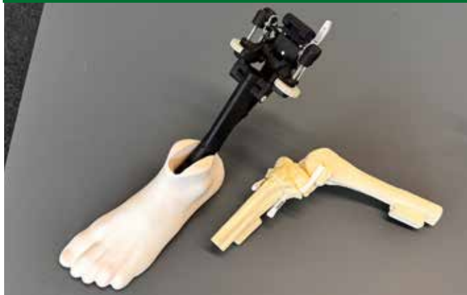
Begin by attaching the knee model's tibia to the Tibial Shaft Mount
