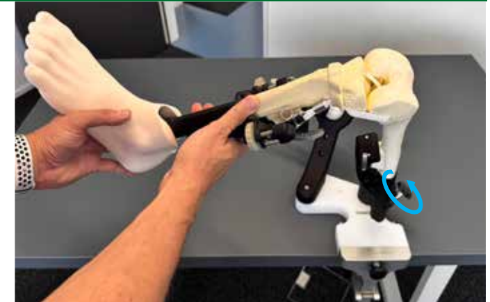
Loosen the hip joint's star knob, then perform leg movements to confirm the range of motion
