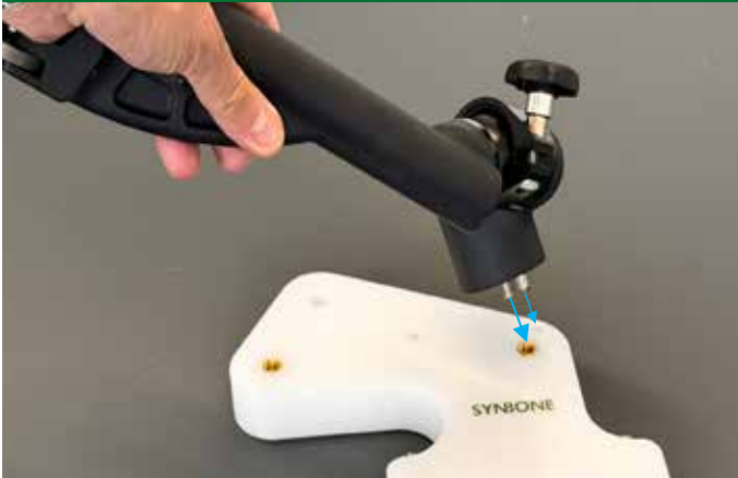
Attach the Hip Joint Base to the Base Plate...
