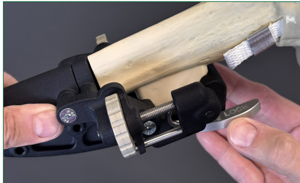
Place the femur and tibia notch's distal groove into the Notch Holder. [For details follow user manual]
